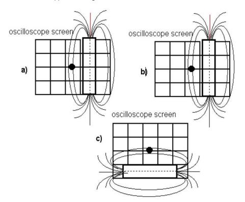
Repeat bringing the magnet to the screen several times, always keeping the same orientation of the magnet. You should notice that when you bring the magnet closer the electron beam moves in some direction; that is it deflected from its original position. Observe the deflection of the spot and record this observation in sketch a) on
