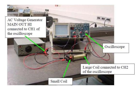
Set the AC generator to a sine wave (push the button on the top right in) of 1000 Hz (push the MULT 100 button in and set the Frequency to 10). Use MAIN OUT HI and turn the AMPLITUDE to maximum (all the way clockwise) if you are using the coils with metal ends, or, if you are using the coils with the black plastic ends set the AMPLITUDE about halfway. Set the oscilloscope to:
